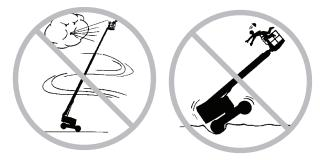
Use extreme care and slow speeds while driving the machine in the stowed position across uneven terrain, debris, unstable or slippery surfaces and near holes and drop-offs. Do not drive the machine on a slope that exceeds the maximum uphill, downhill or side slope rating of the machine. Slope rating applies to machines in the stowed position.
